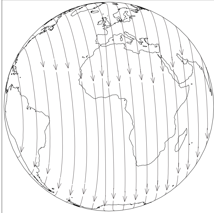
Figure 3.3: Streamfunction for the test case of a dipole magnetic field with instantaneous pole at [\phi_0, \theta_0] = [0, 45N] and rotating perpendicular to the equatorial plane and parallel to the \phi_0 = 0 longitude line at a constant angular velocity \omega = 1^\circ/\text{yr} , with k_0 = 0.1 .
