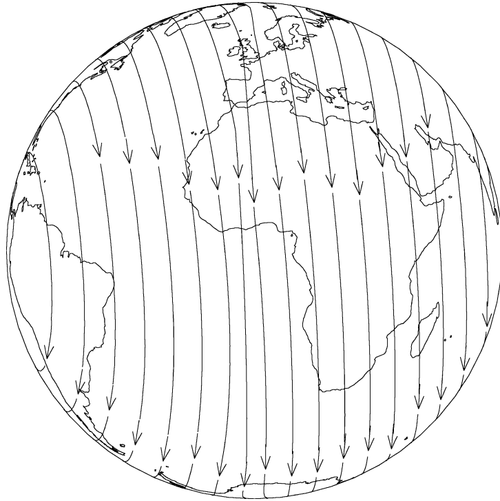
Fig. 2. Streamfunction for the test case of a dipole magnetic field with instantaneous pole at [\phi_0, \theta_0] = [0, 45^\circ \text{N}] and rotating perpendicular to the equatorial plane and parallel to the \phi_0 = 0 longitude line at a constant angular velocity \omega = 1^\circ/\text{year} , with k_0 = 0.1 .
