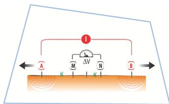
$$\rho_a = K \frac{\Delta V}{I} \quad \text{avec} \quad K = 2\pi \left( \frac{1}{MA} - \frac{1}{MB} - \frac{1}{NA} + \frac{1}{NB} \right)^{-1}$$
