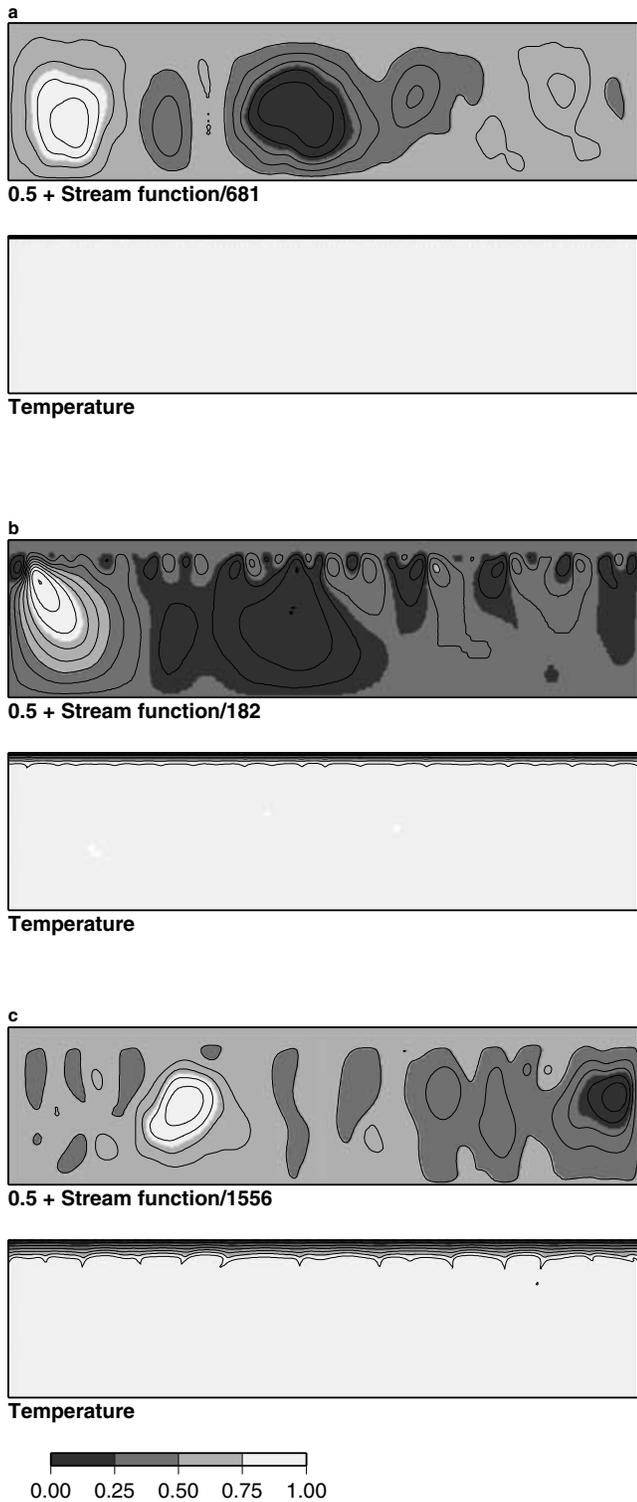
Figure 3. Stream function and temperature fields for simulation 15 of set B ( $Ra_i = 1.58 \times 10^8$ ,  $b = 14.80$  and  $H = 8.10$ ), at (a)  $t = 6.55 \times 10^{-4}$ , (b)  $t = 9.54 \times 10^{-4} = \tau_0$  and (c)  $t = 3.84 \times 10^{-3}$ . The legend is the same as for Fig. 2.
