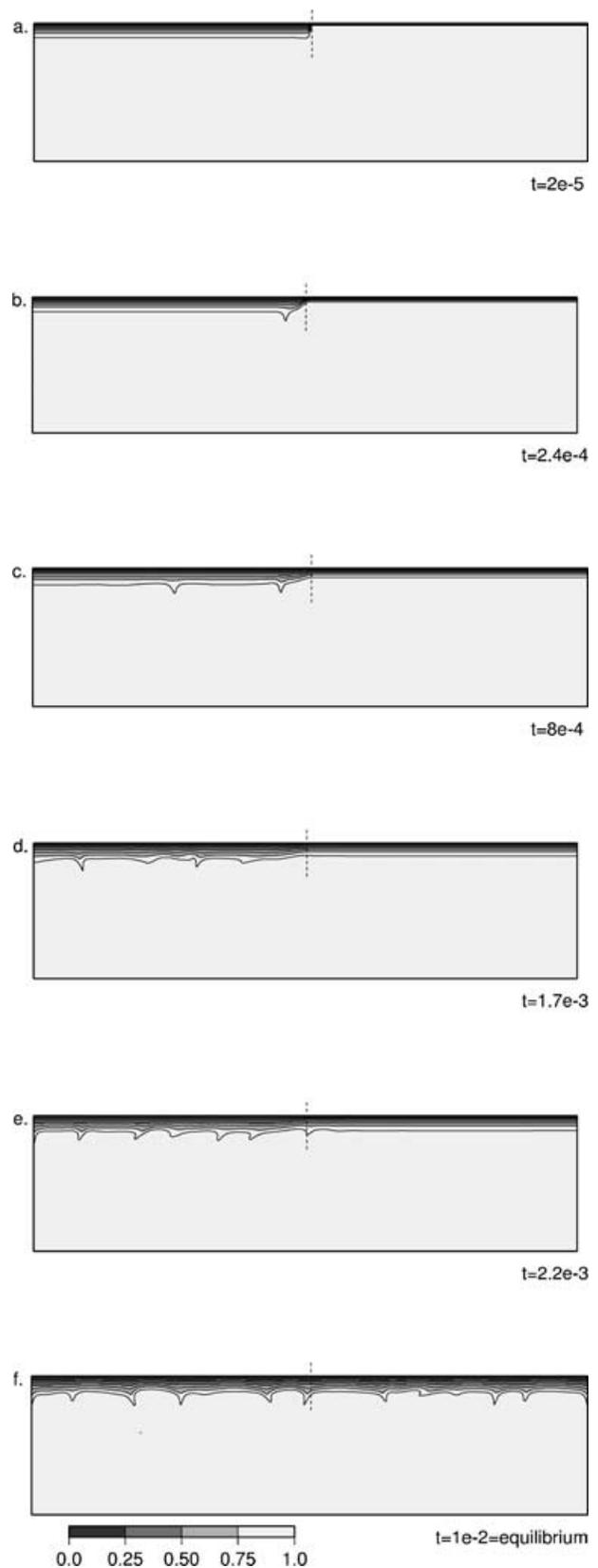
**Figure 12.** Temperature fields at different times obtained for the simulation with a transform fault: (a) the initial temperature field (a lithosphere of age  $t_{\text{erf}} = \tau_0$  on the left side and of age  $t = 0$  on the right side), (b) at  $\tau'_0 < t < \tau_2$ , (c) at  $t = \tau_2$ , (d) at  $\tau_2 < t < \tau_3$ , (e) at  $t > \tau_3$ , and (f) at thermal equilibrium ( $t \gg \tau_3$ ).
