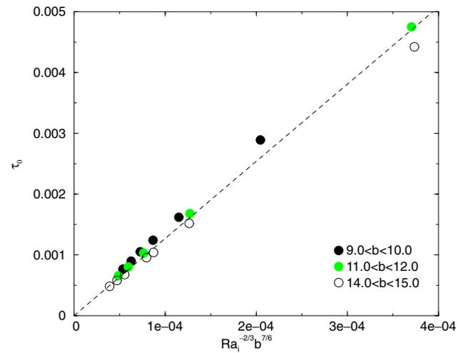
**Figure 7.** Age of first dripping instability obtained for set  $B$ ,  $\tau_0$ , is plotted as a function of  $Ra_i^{-2/3} b^{7/6}$ . This scaling is obtained with the assumption that marginal stability controls  $\tau_0$ . Black circles are drawn for simulations with  $9.0 < b < 10.0$ , grey circles for simulations with  $11.0 < b < 12.0$  and open circles for simulations with  $14.0 < b < 15.0$ . A linear regression (dashed line) yields a slope of 12.70.
