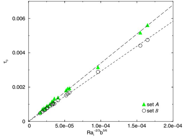
**Figure 9.** The age of first dripping instability,  $\tau_0$ , is plotted as a function of  $Ra_i^{-2/3} b^{5/6}$ . This scaling is obtained with the assumption that perturbations growth rates control  $\tau_0$ . Grey triangles are drawn for simulations with two initial single point perturbations (set  $A$ ) and circles for simulations having an initial temperature field randomly perturbed (set  $B$ ). The regression slopes are respectively of 33.93 and 29.20.
