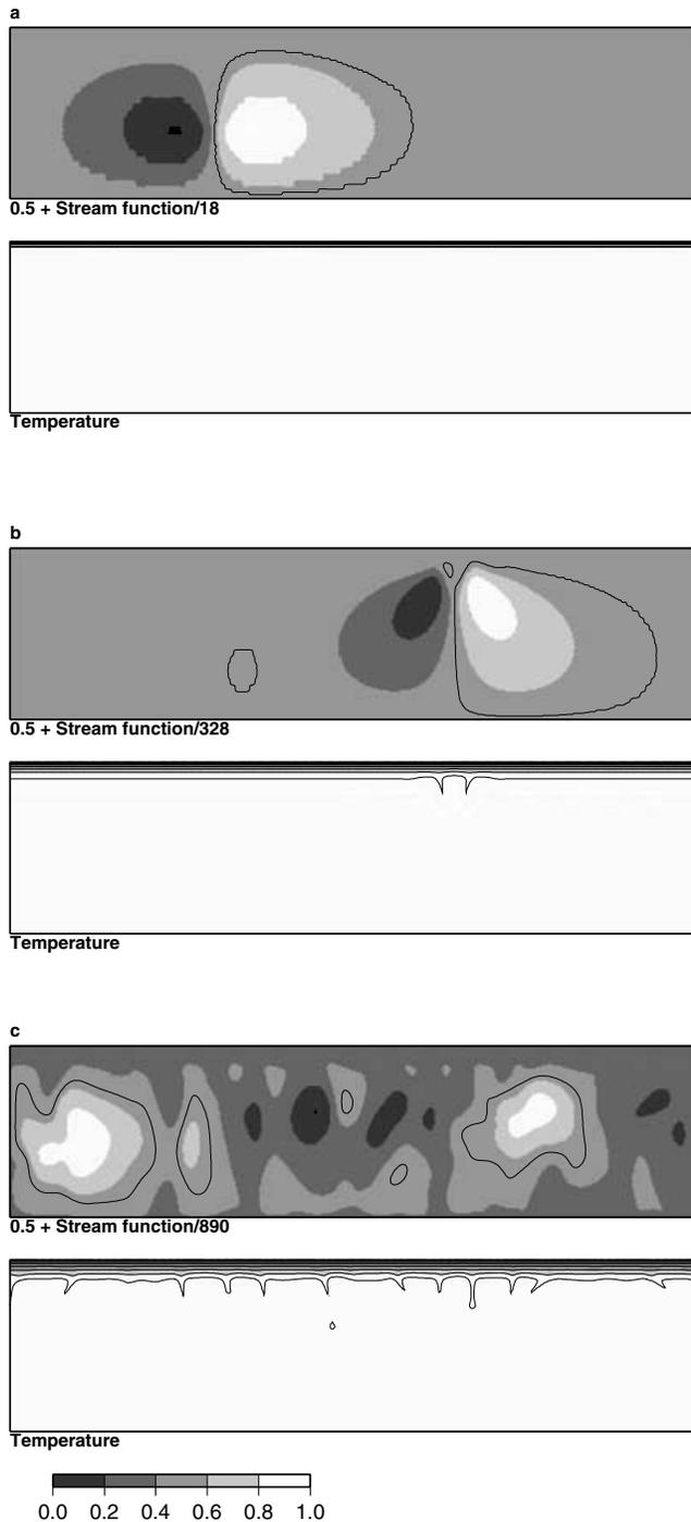
**Figure 2.** Stream function and temperature fields for simulation 15 of set *A* ( $Ra_i = 1.58 \times 10^8$ ,  $b = 14.80$  and  $H = 8.10$ ), at (a)  $t = 1.32 \times 10^{-5}$ , (b)  $t = 1.16 \times 10^{-3} = \tau_0$  and (c)  $t = 2.64 \times 10^{-3}$ . Variables are dimensionless. The stream function is normalized to be bracketed between 0.0 and 1.0. The black lines in temperature fields are isotherms.
